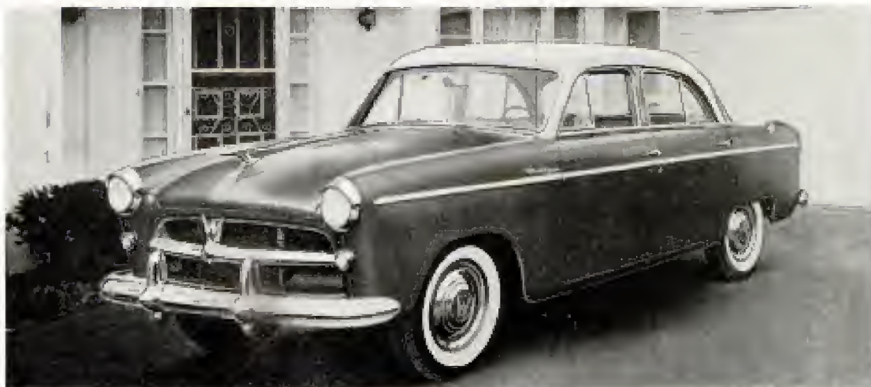
Willys Ace has a new grille, larger engine, restyled interior. Automatic transmission is available this year
